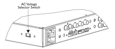
wall outlet, check whether the AC mains voltage and frequency is compatible with this product (see rear panel of product). Whenever the specified voltage or your AC plug should not match the local conditions, do NOT plug the
