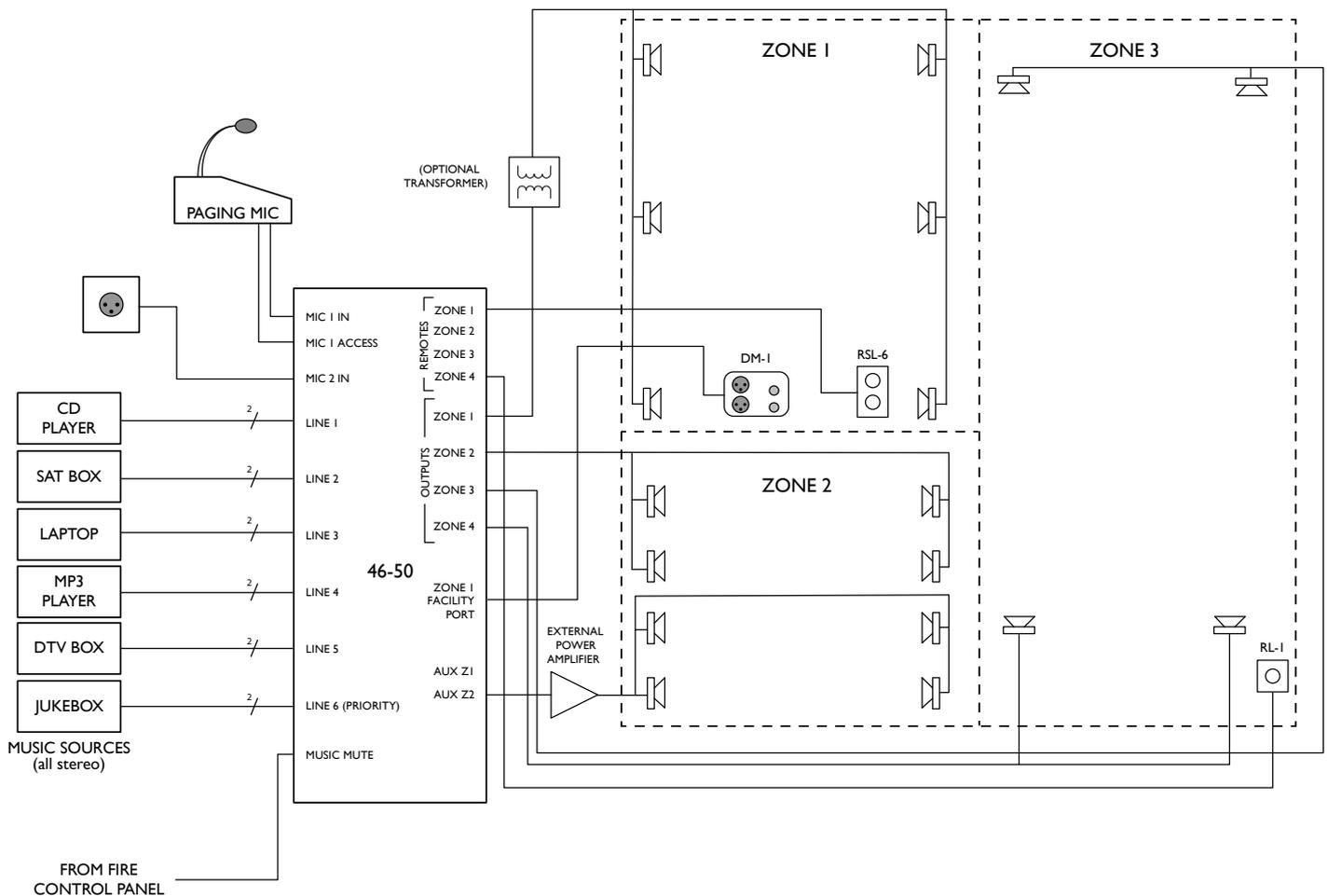
The example shows how the 46-50's various features may be used in an installation situation based on three distinct building areas.
