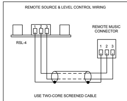
Use two-core (RSL-4/RSL-4A or RL-1/RL-1A) or single-core (RL-1/RL-1A only) screened cable to connect the remote level plate. The maximum recommended cable length is 100 m.
