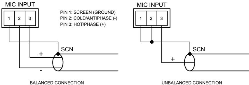
15V phantom power is available at the mic input, and is activated by setting internal jumper J1 to the ON position. See "PCB layout diagrams" on page 30 for further
