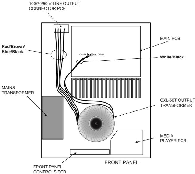
5. The primary winding of the transformer is terminated in a two-pin Molex-type connector. This should be plugged into the header marked CN15B on the main PCB. See “PCB layout diagrams” on page 30 for location.
