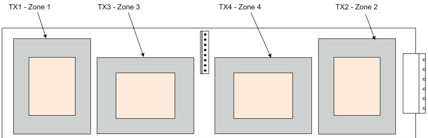
CXL-4160 transformer module PCB assembly
