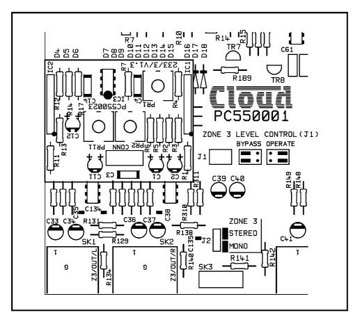
3. Locate the 10 pin male connector positioned adjacent to the respective output zones. This should have each end pair of contacts shorted by single circuit jumpers. Remove these two jumpers.
