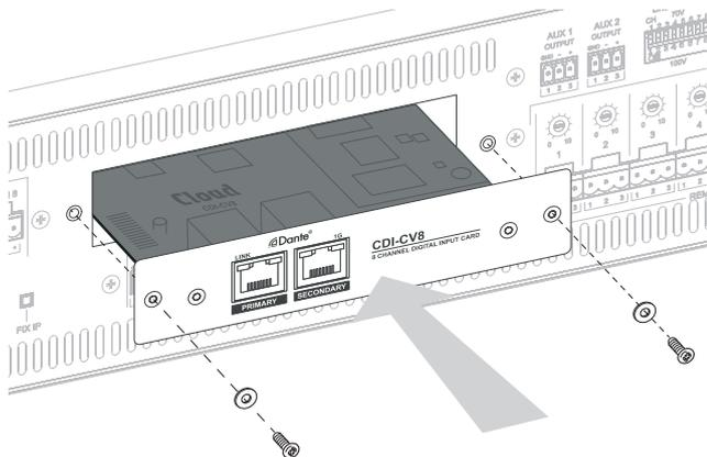
6. Secure the card in place with the two screws removed in Step 4. (Note these are the only fixings the card requires.)
