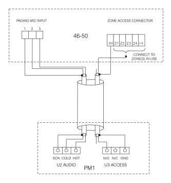
Note that the default factory setting routes **MIC I** to all four zones at all times. In order for **MIC I** to function correctly with a paging mic, internal jumpers J23 (Zone I), J22 (Zone 2), J21 (Zone 3) and J20 (Zone 4) should be removed to enable the **PAGING ACCESS** connector. See page 24 for jumper locations.
