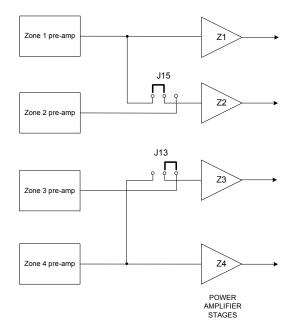
Selection of parallel operation is made by moving internal main PCB jumpers J15 (Zones 1 & 2) and/or J13 (Zones 3 & 4) from their default setting. See page 24 for locations of PCB jumpers.
