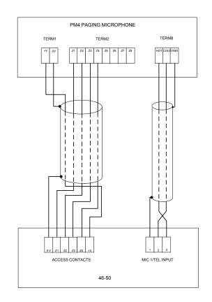
Note that the default factory setting routes **MIC I** to all four zones at all times. In order for **MIC I** to function correctly with a paging mic, internal jumpers J23 (Zone I), J22 (Zone 2), J21 (Zone 3) and J20 (Zone 4) should be removed to enable the **PAGING ACCESS** connector. See page 24 for jumper locations.
