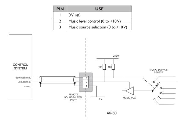
**NOTE:** If the control voltage source is not isolated from the power earth, there is a small risk of creating a 'ground loop' by linking the mixer technical ground (0V) to the ground (0V) of the equipment supplying the control voltages. To minimise this risk, we suggest that all pieces of equipment be in close proximity, and supplied from the same power outlet.
