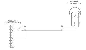
An unbalanced source may also be connected; the use of balancing transformers is recommended
