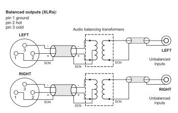
If transformers are not available, a balanced source may feed an unbalanced input directly as long as care is taken over how the connections are made. A variety of design techniques are in use to implement balanced outputs in audio equipment,
